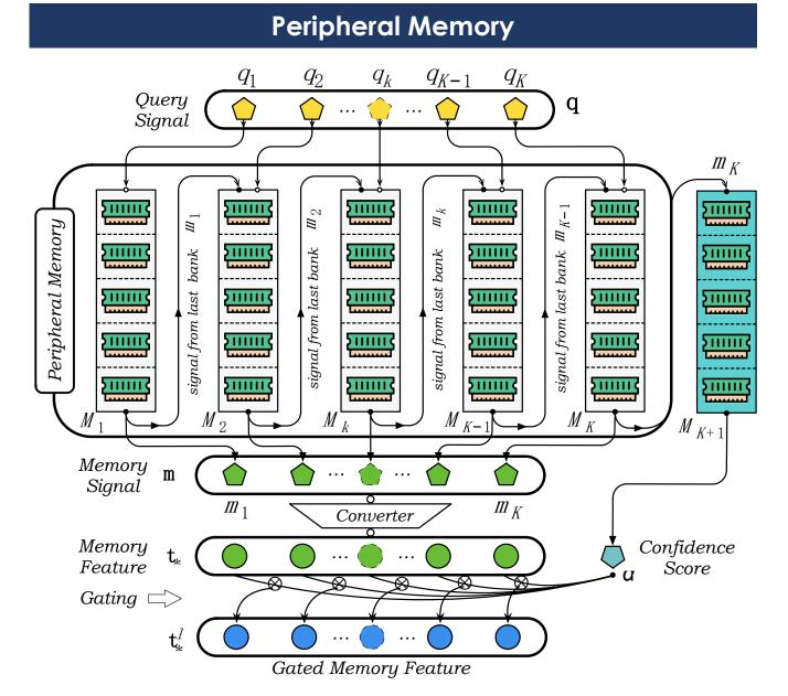
The peripheral memory is composed of two components: <u>memory</u> <u>banks to store data</u> and <u>the confidence bank to evaluate the relevance</u> between the query feature and the retrieved information. The number of memory banks determine the memory bandwidth. Moreover, these banks are interconnected with each other, i.e., the output of the one bank will be regarded as the input of the next one.
