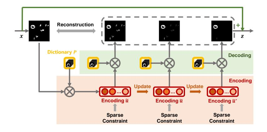
In each VARS block, we iteratively optimize the sparse reconstruction using ISTA (LISTA)
