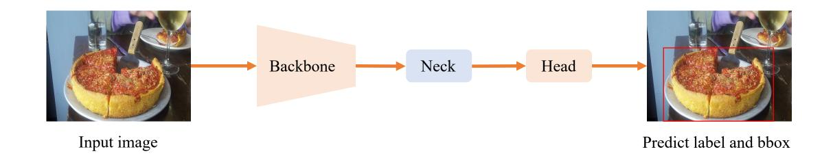
✓ The performance of object detection network heavily depends on the feature extraction backbone.
