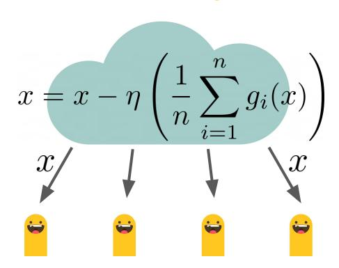
Server accumulates gradients and computes new parameters
