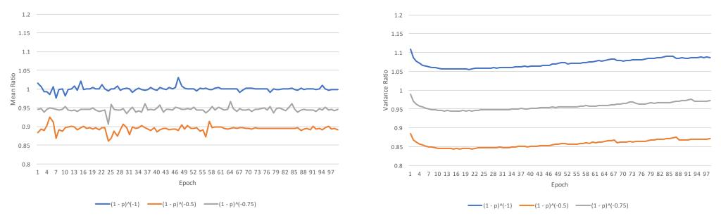
Changes of Mean (left) and Variance (right) when applying various rescaling factors. Blue: Dropout Grey: Jumpout
