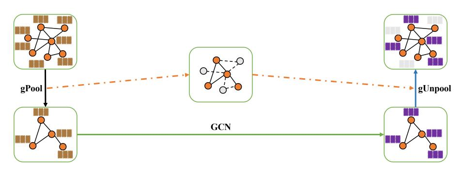
gUnpool layer uses position information from gPool layer to reconstruct original graph structure.
