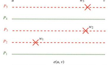
Figure 2: A faulty vertex set  $F = \{w_1, \dots, w_{\hat{f}}\}$  of size  $\hat{f}$  can invalidate at most  $\hat{f}$  paths out of f vertex-disjoint paths between endpoints u and v of an edge e(u, v). Here f = 5 and  $\hat{f} = 3$ .
