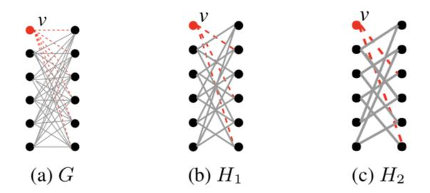
Figure 1: 1-FT cut sparsifiers of G:  $H_1$  and  $H_2$ . (a) G with 36 edges and edge weight 1. (b)  $H_1$  with 18 edges and edge weight 2. (c)  $H_2$  with 12 edges and edge weight 3. Without loss of generality consider that v is faulty. The *Min-Cut* of  $G - \{v\}$  is 5, while the *Min-Cut* of  $H_1 - \{v\}$  and  $H_2 - \{v\}$  are 4 and 3, respectively. Then  $H_1$  and  $H_2$  are 1-FT  $(1 \pm 0.2)$ -cut sparsifier and  $(1 \pm 0.4)$ -cut sparsifier of G, respectively.
