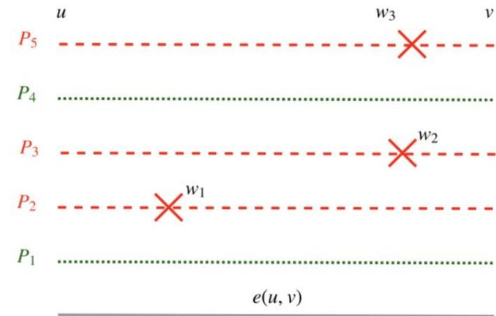
Figure 2: A faulty vertex set  $F = \{w_1, \dots, w_{\hat{f}}\}$  of size  $\hat{f}$  can invalidate at most  $\hat{f}$  paths out of  $f$  vertex-disjoint paths between endpoints  $u$  and  $v$  of an edge  $e(u, v)$ . Here  $f = 5$  and  $\hat{f} = 3$ .
