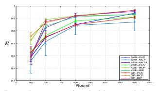
Figure 3. Learning curves for each of the nine methods on Oracle 9. Each curve shows the probability of detection  $(P_d)$  at a fixed false alarm probability  $(P_{fa} = 0.05)$  as a function of the number of rounds of active learning. Except for SVM-MCP, the active methods clearly outperform passive. KDE-MCP reaches 90%  $P_d$  at round 100, while KDE-PAS doesn't reach this level until after round 300, representing speedup by a factor of three.
