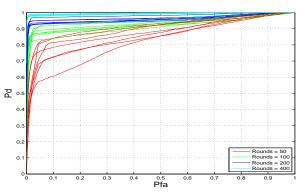
Figure 2. ROC curves on Oracle 7 for GP-MCP, colorcoded by number of rounds (r). For each value of r, seven trials were conducted to assess variability.
