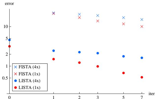
Figure 3. Code prediction error as a function of number of iterations for FISTA (crosses) and for LISTA (dots), for  $m = 100$  (red) and  $m = 400$  (blue). Note the logarithmic scales. iter = 0 corresponds to the baseline trainable encoder with the shrinkage function. It takes 18 iterations of FISTA to reach the error of LISTA with just one iteration for  $m = 100$ , and 35 iterations for  $m = 400$ . Hence one can say that LISTA is roughly 20 times faster than FISTA for approximate solutions.
