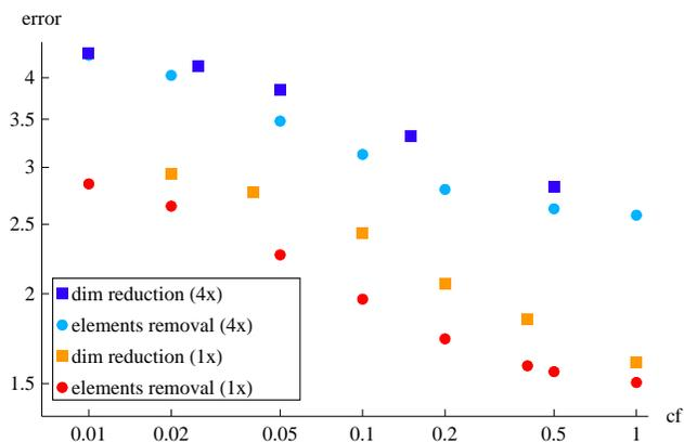
Figure 4. Prediction error for LISTA with one iteration as a function of fraction of operations  $c_f$  required relative to a full  $S$  matrix. The matrix is reduced using a low rank factorization, or by removing small elements.
