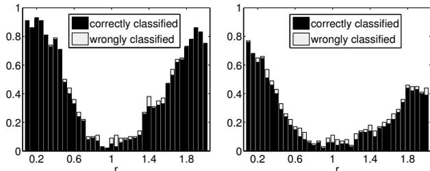
Figure 2. For each value of  $r$  (i.e. for each kind of noise) we simulated 100 instances of an ARMA(2,2) process. The graphs show the proportion of correctly and wrongly classified time series depending on  $r$ . Because Gaussian ARMA processes are symmetric in time, the method has to fail for  $r \approx 1$ . The left panel shows our method using the HSIC independence test, for the right one we used a  $\chi^2$  independence test instead, which results in a worse performance.
