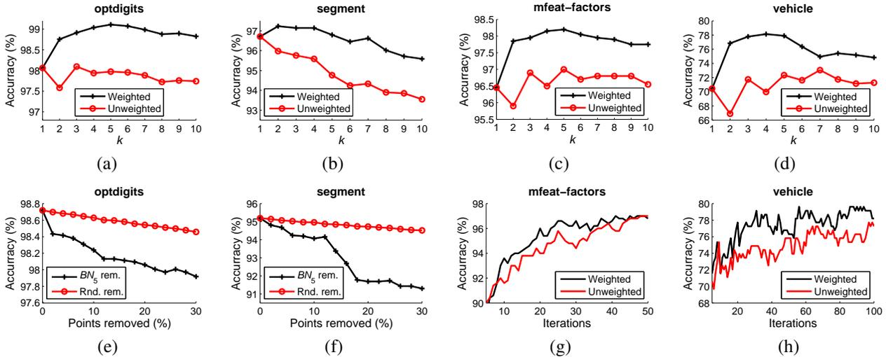
Figure 4. (a–d) Accuracy of  $k$ -NN classifier with and without the weighting scheme. (e, f) Accuracy of SVM with RBF kernel and points being removed from the training sets by decreasing  $BN_5$ , and at random (averaged over 20 runs). (g, h) Accuracy of AdaBoost with and without the weighting scheme: (g)  $k = 20$ , (h)  $k = 40$ .
