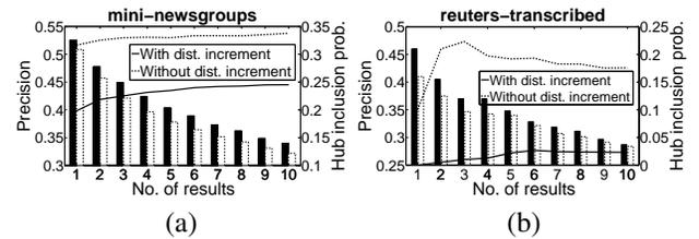
Figure 7. Precision with (solid bars) and without (dashed bars) the distance increment scheme: (a)  $k = 10$ , (b)  $k = 1$ . Inclusion probability of hubs is also plotted (against the right vertical axes) with (solid line) and without (dashed line) the increment scheme.
