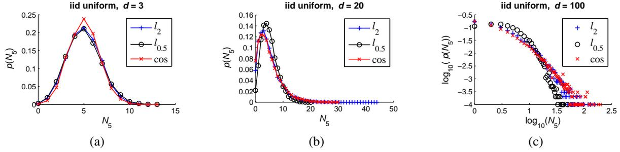
Figure 1. Distribution of 5-occurrences for Euclidean,  $l_{0.5}$ , and cosine distances on iid uniform random data sets with dimensionality (a)  $d = 3$ , (b)  $d = 20$ , and (c)  $d = 100$  (log-log plot).
