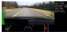
Figure 6: Screenshot of the simulator in interactive mode. See Section 7.1 for explanation of the performance metrics. The green area on the left is cut away because of the stereographic transformation. The highlighted white rectangle below the horizon is the area which is sent to the CNN.
