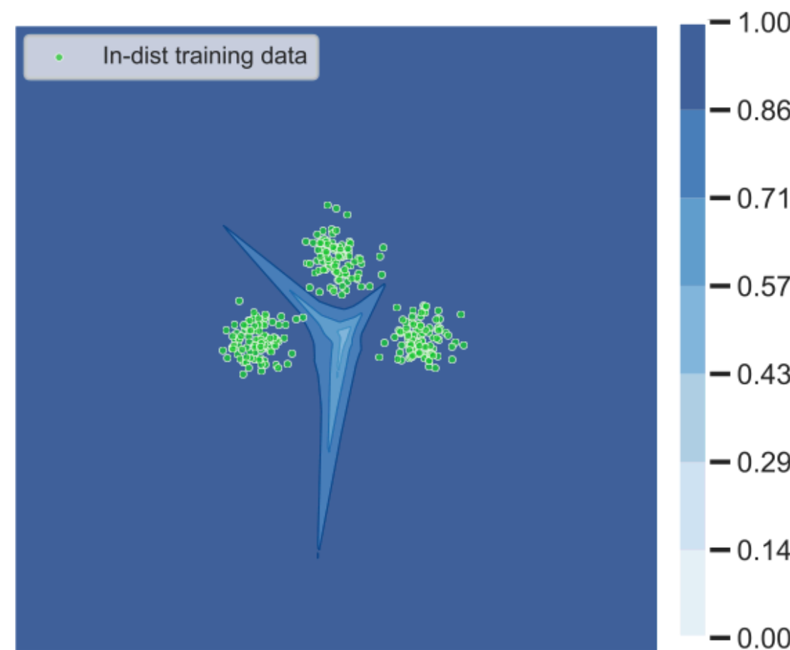
Maximum Softmax probability over ID categories when the network is trained with only ID data (green)
