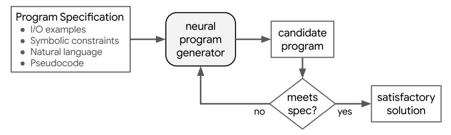
Sample candidate programs from the neural generator conditioned on the spec
